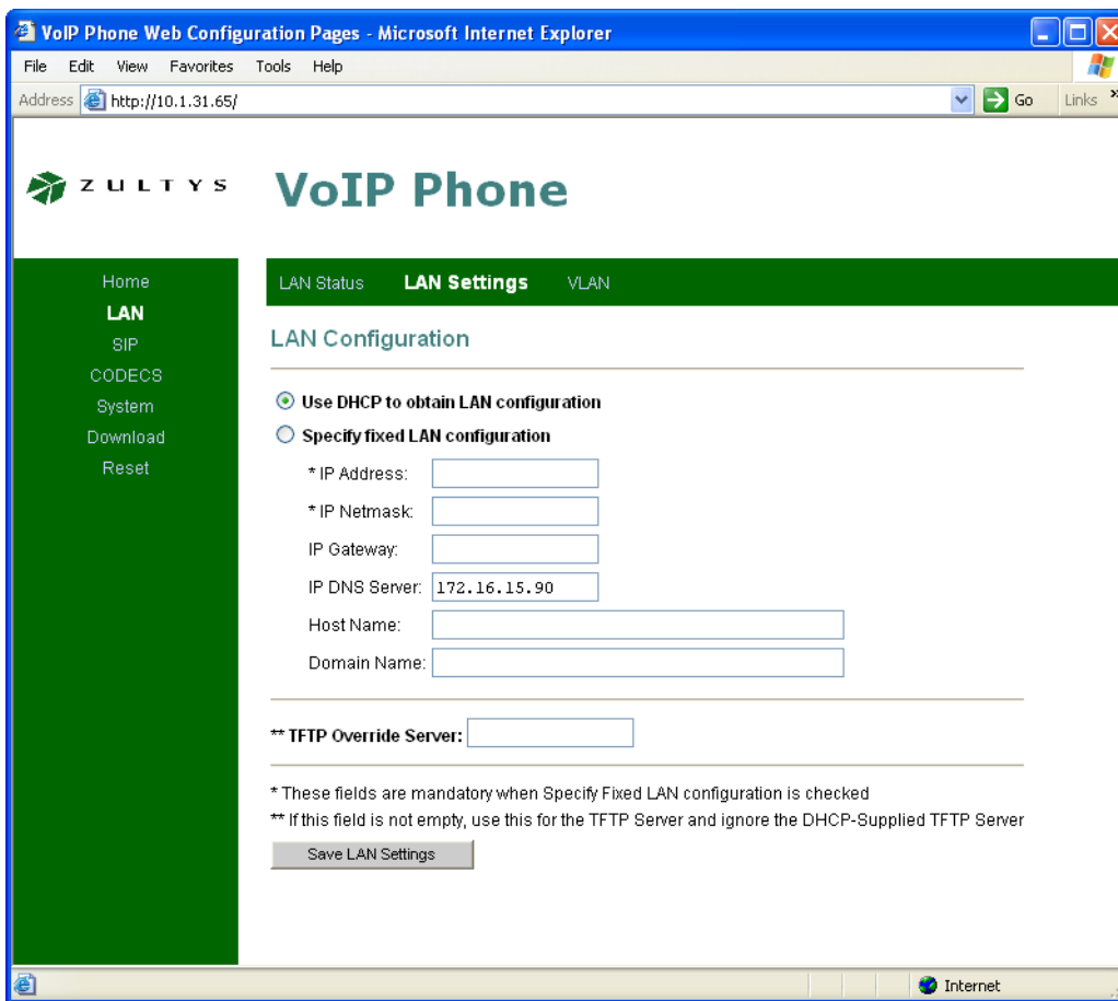
Figure A-3 LAN Configuration panel
