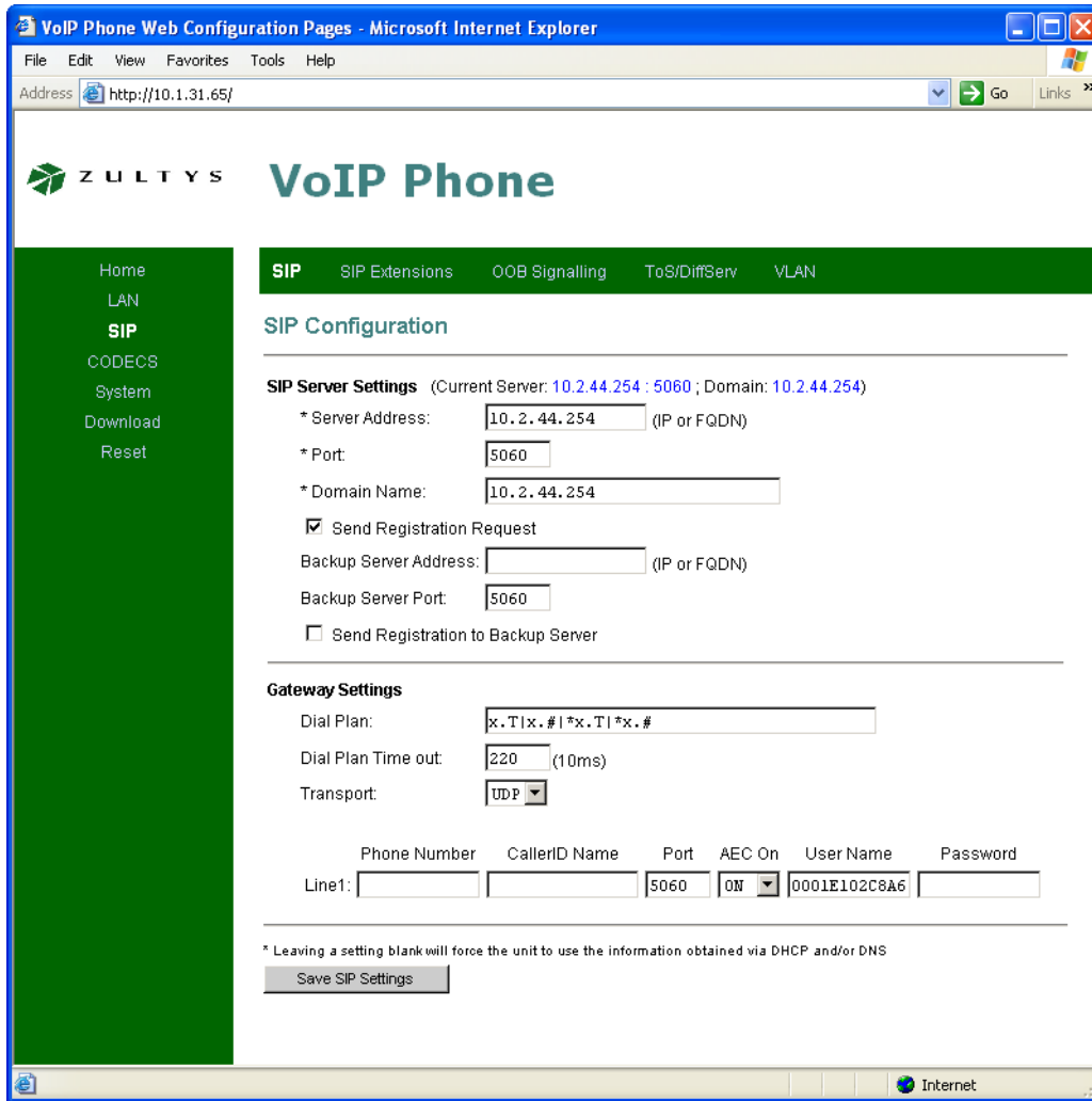
Figure A-5 SIP Configuration panel
