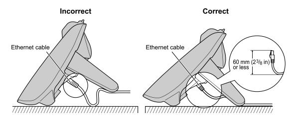
• Use a straight CAT 5 (or higher) Ethernet cable (not included) that is 6.5 mm (1/4 in) in diameter or less.
