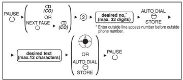
Similar to the above procedure, when storing other types of buttons (CO buttons, feature buttons, etc.), the displayed text for the Self Labeling LCD Display can be assigned.
