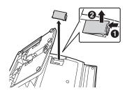
3. Plug the flat cable into the connector (♠), then bend the cable slightly as shown (♠).
