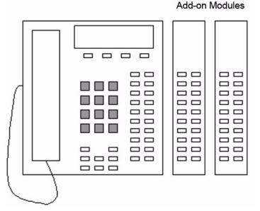
It is possible to increase the number of function keys by connecting the DSS console having 60 buttons to the system and associating it to an IPT.
